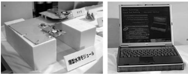
Fig. 7 A piezoelectric pump water cooling module ( left ) for a fuel cell in a laptop computer.[Courtesy by NEC]
